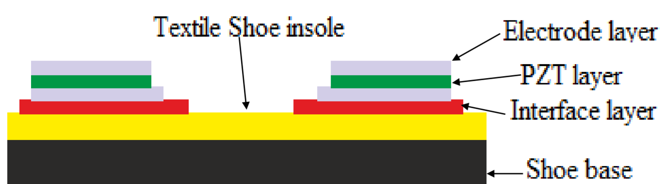
Figure 5 : Schematic of the piezoelectric shoe-insole energy harvester structure
